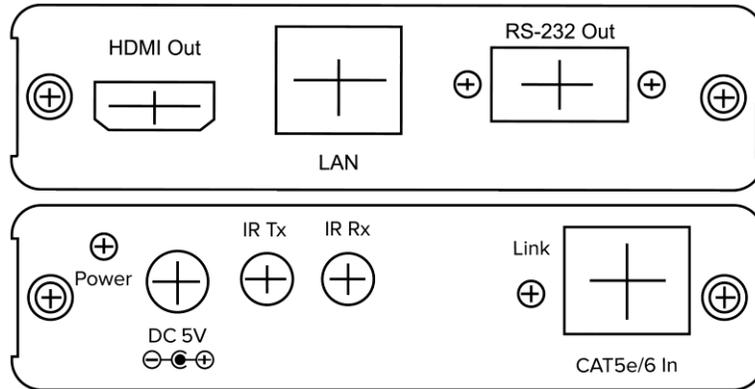
1. At the remote location, connect the Cat.5e/Cat.6 cable to the Receiver's CAT5e/6 In port. Ensure that the RJ45 connector is securely locked into the receiver's port.
