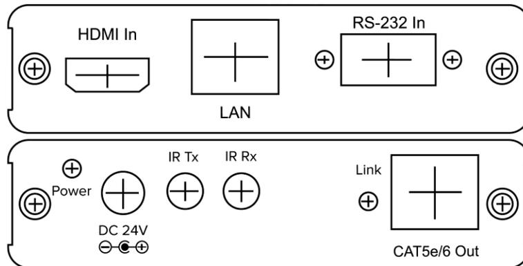
1. Connect the HDMI source device's output to the HDMI IN port of the 1T-CT-653 Transmitter, using an appropriate HDMI cable, (1 Meter (~3') in length for 12 bit signals, 10 meters (~33') for 8 bit signals).
