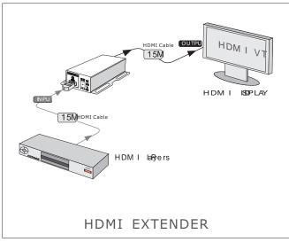
The SB-6225 is a transmission of HDMI over CAT5/6 category cable wires for 30M length which supports HDMI 480i/P, 576i/P,720P(50/60Hz), 1080i and 1080p(50/60Hz). The best install between the HD DVD player and HDMI Display monitor with 15M HDMI cable each.
