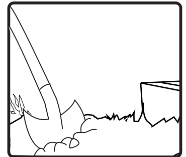
2. For in-ground installation, dig a hole 6 - 8" in diameter and 8" deep in the precise location where the speaker will be placed.
