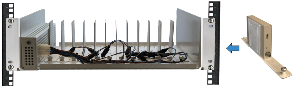
Figure 14. Add Carrier with Mini-Converter into slot in DRM2 Frame
