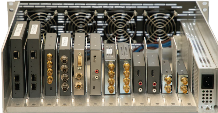
Figure 1. DRM2 with twelve Mini-Converters mounted on Carriers
