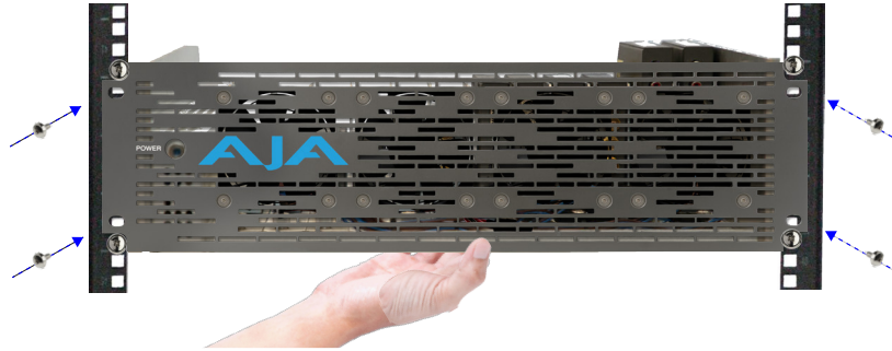
Figure 19. Attaching an Active Faceplate
