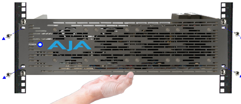
Figure 20. Removing an Active Faceplate
