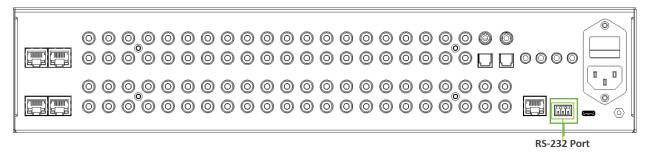
Wiring for this port uses a 3-pin terminal block connector to DB9, where only pins 2, 3, and 5 are used. If the control devices do not have a DB9 port, a USB to DB9 adapter may be required.
