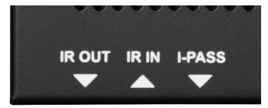
IR OUT - This port is designed to accept an IR Emitter
