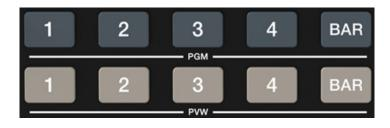
**PGM**: Use the PGM buttons to select which source is being used as the two HDMI Program outputs.
