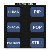
• **LUMA:** Removes the color black from the background of the PVW image and overlays the remaining imager on top of the PGM output. Typically used to place a watermark, logo, text, or subtitles on the PGM output
