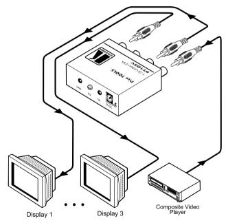
Figure 4: Connecting the PT103V 1:3 Video DA
