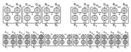
Figure 7: Configuring as a 3 x 1:2 RGB distributor
