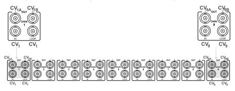
Figure 3: Configuring as a 9 x 1:2 Composite Video Distributor
