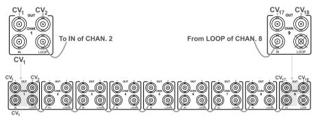
Figure 4: Configuring as a 1:18 Composite Video Distributor
