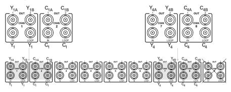
Figure 5: Configuring as a 4 x 1:2 s-Video (Y/C) Distributor
