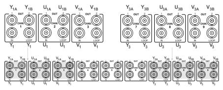
Figure 6: Configuring as a 3 x 1:2 Component Video (YUV) Distributor
