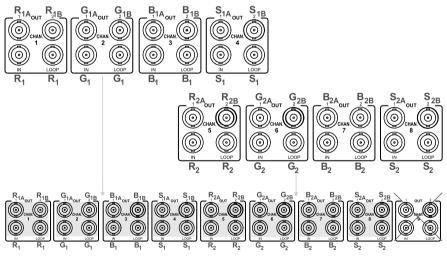
Figure 8: Configuring as a 2 x 1:2 RGBS distributor
