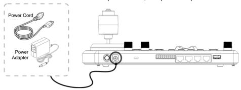
■ POE power supply: Use Ethernet cables to connect POE switch and IP port of VS-KB30, and press the POWER button
