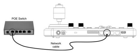
[Note] RJ45 ports of RS232 and RS422 do not support POE. Please do not connect with POE-powered network cables
