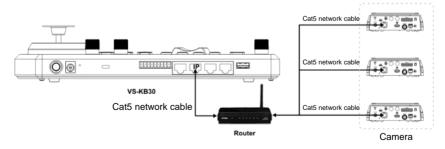
1. Use network cables to connect VS-KB30 and IP camera to the router
