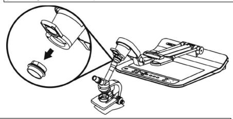
For eyepieces of Ø28 mm or Ø31 mm, fit one microscope adapter with the greatest diameter along with another appropriate one.
