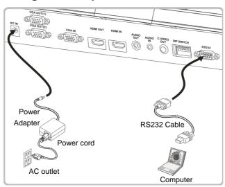
After connecting to the RS232 cable, you can use RS232 commands to control PS752.
