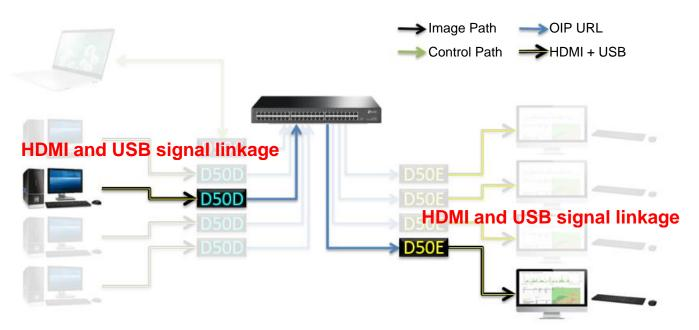
6.2.2 D50D decoder has a UI interface for easily operating KVM
