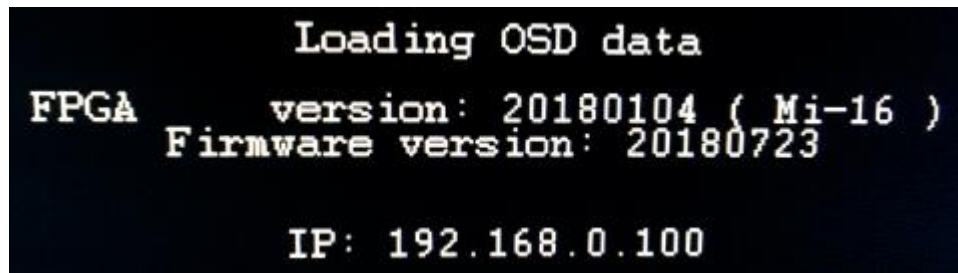
Figure 6: FPGA/FW version and IP address of the unit will be displayed for about 5 seconds
