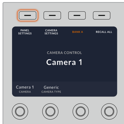
Press the 'settings' soft button on the LCD home screen to access all the camera control panel's settings
