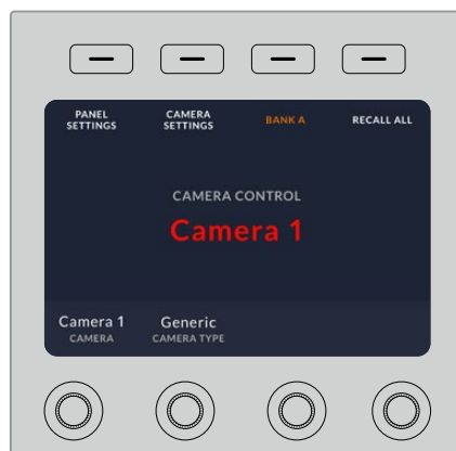
The camera name and number on the LCD home screen shows the camera currently selected for each CCU
