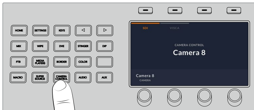
To use VISCA PTZ control, press the 'camera control' button and select VISCA by pressing the VISCA soft button.
