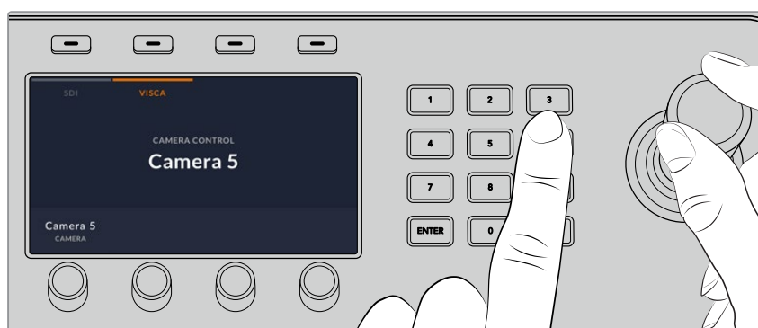
Select the camera you want to control and use the joystick to pan, tilt and zoom
