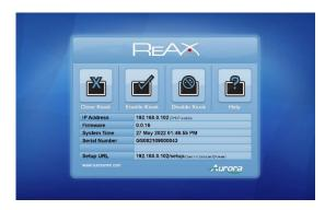
longer be displayed. At this point, this page can be accessed from a web browser by pointing to http://**[IP Address]**/home where [IP Address] is the IP address of the RXT device. This page can be restored to the default by setting the 'Kiosk Home Page' found in the <u>Network Settings</u> page to 'http://localhost/home'.
