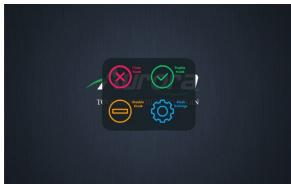
**Disable Kiosk:** Click to and disable the Kiosk mode of the RXT device. This will expose the user controls of the underlying Android system. By default, the Kiosk is Enabled.
