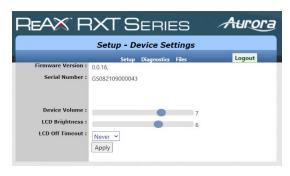
**LCD Off Timeout:** Use the drop-down box to select the desired screen timeout. The screen will go black and display only the date and time when the selected time expires beyond the last user interaction with the RXT device. The screen will wake up when the LCD is touched. Select 'Never' to keep the display on full-time.
