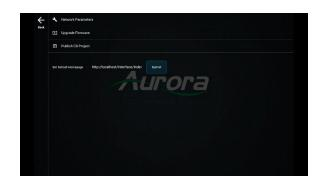
**Publish CS Project:** Browse for a valid Core Studio project (\*.acs) file either locally on the RXT device or from a USB plugged into the device. This will replace any currently loaded project and reboot the RXT device.
