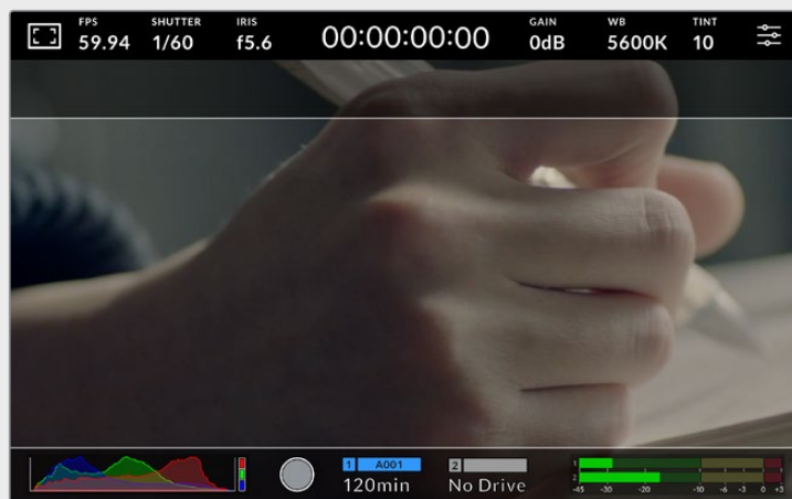
The LCD touchscreen with 2.40:1 frame guides enabled
