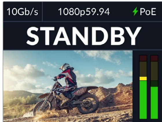
When power and video is connected, the PoE indicator will illuminate green, followed soon after by the video image and 'standby' indicator
