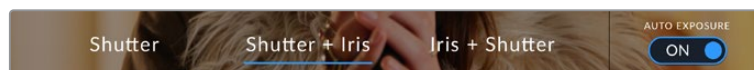
While in the shutter menu, tap 'auto exposure' to access shutter based auto exposure modes
