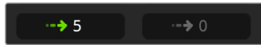
Click on the delay indicator below the level input knob to open the delay control.
