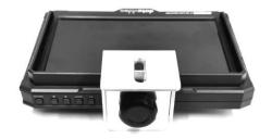
If you intend to mount a small box camera or webcam directly to the TTL-100, attach the aluminium monitor bracket (Item A) and the aluminium camera bracket (Item B) to the TLM-700 monitor using the large ½ screw (Item D).
