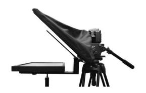
Position the TP-700 in front of the camera lens and pull the draw cord to secure the cloth Snood / Hood, item I, around the camera lens and to shut out light from the camera side.
