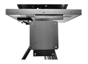
If your monitor has a 100MM VESA mount, first attach the VESA adapter plate, item T to the vertical mounting rail, item S using the 12mm M4 screws, Item CC, then attach the monitor to the VESA adapter plate using the 8MM M4 screws, item CCC.
