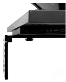
Attach the talent monitor vertical mounting rail, item S, to secure the lower part of the ENG Prompter Frame item B using the M4 screws, item BB.
