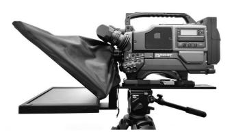
14. Pull the draw cord to secure the cloth Snood / Hood, **item I**, around the camera lens and to shut out light from the camera side.
