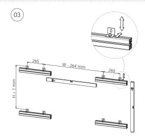
Screw now the brackets with Profile(s) on the wall. Line-up the profile(s) by adjusting the wallbrackets (2).
