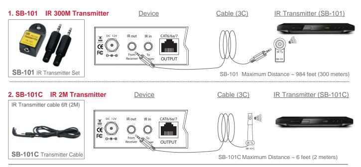
\*\*\* When you plug the External IR extender into the switcher, the front panel IR transmitter remains active. \*\*\*
