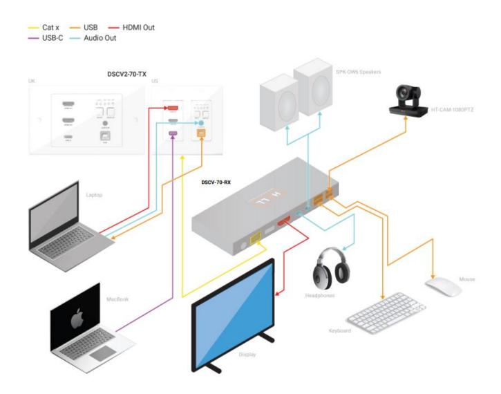
The above application demonstrates the possible connections for the DSCV2-70-TX and DSCV-70-RX. In this application the laptop not only shares video via HDMI, but also receives video from the HT-CAM-1080PTZ via the USB host, allowing for the laptop to be used as a soft codec.
