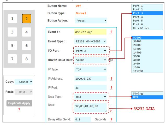
**Figure 7c7b:** Example RS232 command info collected from Owner's Manual of the controlled device. For HEX data type, KD-WP8 requires each byte to be separated by a comma, without any spaces between byte.
