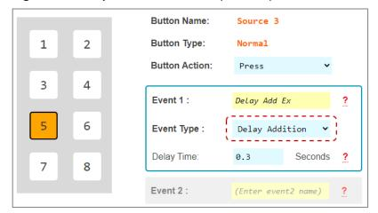
Figure 7c4: IR KD-CX/922 Event example and options. IR Data is pasted from a Pronto Hex Sheet. See figure 7c4b.
