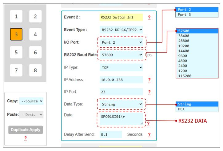
**Figure 7c6b:** Browsing Key Digital's RS232 Database Manager for the command data used in the above example. Identifying the device, Baud Rate, and RS232 Command Data.
