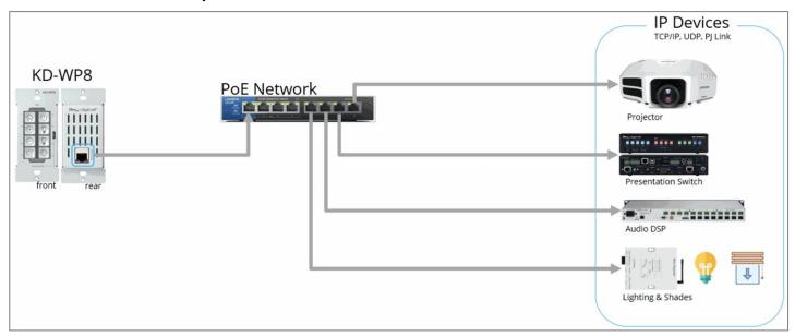
**IP, IR, RS, Relay Control -** For IP Control, KD-WP8 sends commands directly to the devices via the network. For IR, RS-232, and Relay control, KD-WP8 sends command string and burst info to KD Master Controller.
