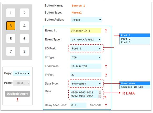
**Figure 7c4b**: Example Pronto Hex IR sheet collected from mfr. The highlighted hex data has been copied and pasted into the Event's Data cell.
