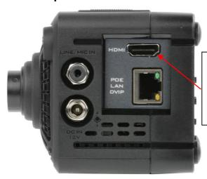
Connect HDMI devices such as TLM series monitors, ShowCast 100, iCast 10NDI, and HDR-80/90. Via an HDMI cable, the HDMI interface will then be able to deliver the camera image to an HDMI display such as an HDMI monitor (TLM series monitors), a switcher (ShowCast 100/iCast 10NDI) or a recorder (HDR-80/90).
