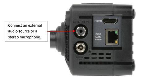
The 3.5mm headphone jack allows you to connect an external audio source using LINE IN or a stereo microphone using MIC IN. The external audio source is embedded in the output video.
