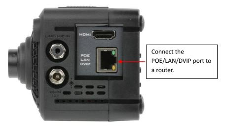
Connect the Ethernet interface to a router. The IP address can be found in <u>Network Info</u> of the OSD menu.
