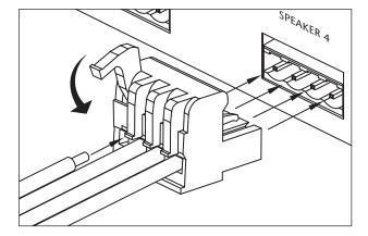
Figure 3 Connecting the Wires
