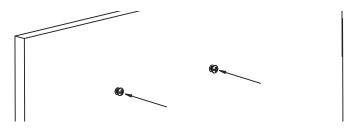
2. Hang the unit to the hanging hooks matching the bracket's hanger keyholes.
