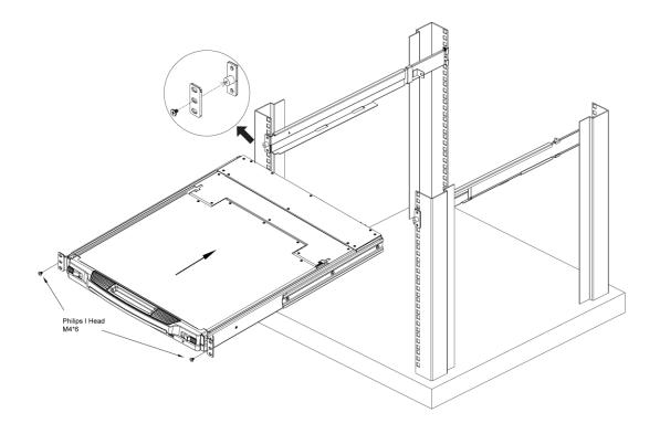
**4.** Stabilize the LCD unit further by screwing an M4\*6 Type I Screw to each of the unit's *rear attachment sliding brackets*.
