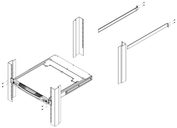
**3.** After the L-shaped brackets are secured, tighten all the screws.
