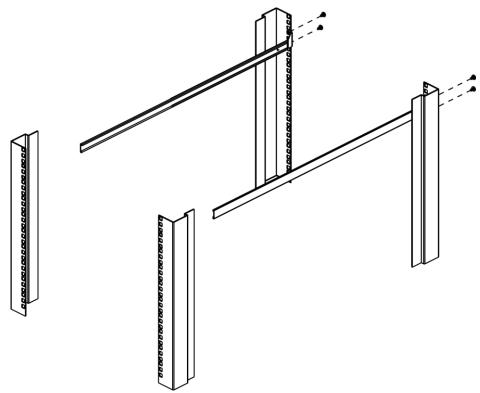
2. While one person inserts the unit into place by sliding its left and right side bars into the left and right L-shaped brackets (on the rack), have a second person screw the front brackets to the rack.
