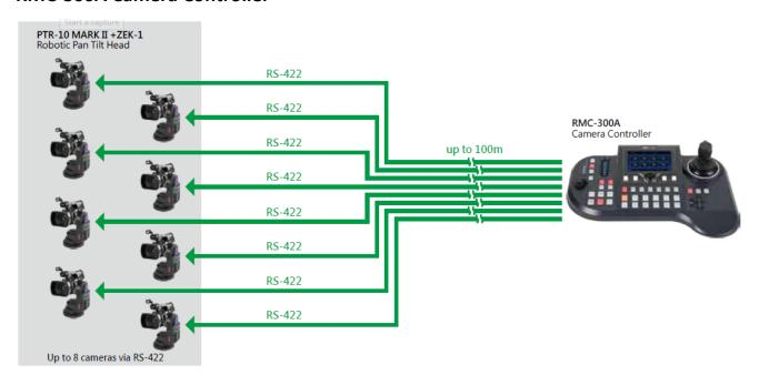
To control the camera mounted on PTR-10 MARK II using the camera controller, first connect one of the RJ-45 ports provided on the controller rear to PTR-10 MARK II's RS-422 IN port via an RJ-45 cable. Then depending on the protocol used, either connect PTR-10 MARK II to the camera via the Remote
