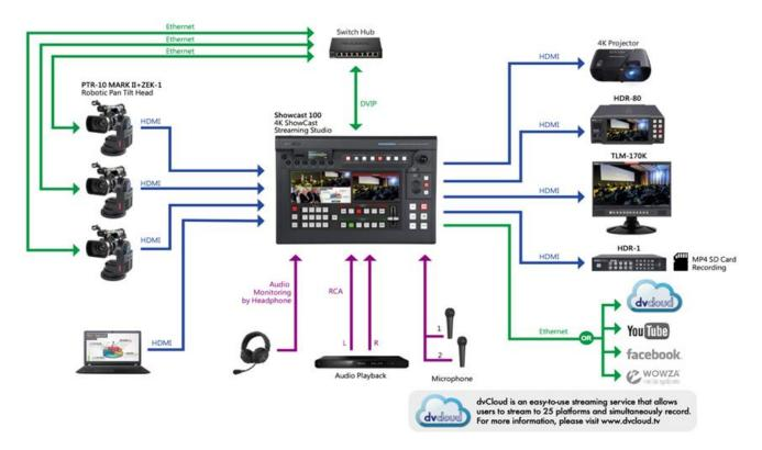
PTR series device usually has a default static IP address of 192.168.100.XXX. Using an RJ-45 Ethernet cable, the unit can be directly connected to a Windows-based computer assigned of an IP address with the same first three octets as the unit's default IP address. The following setup procedure
