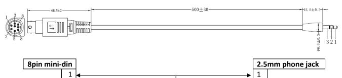
Warning: The 8pin snap-and-lock mini-din connector of the remote cable will be securely fastened once plugged into the Remote port. To remove, use two fingers to gently hold the part of the plug labelled by two arrows then pull the connector outward.
