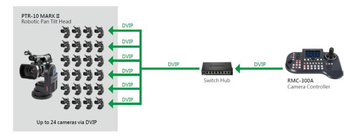
In the second diagram, the Showcast 100 4K ShowCast Streaming Studio communicates with the PTR-10 MARK II devices through a switch hub.
