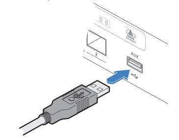
2 Connect an accompanying USB-to-serial converter to a vacant USB socket on the RX unit.
