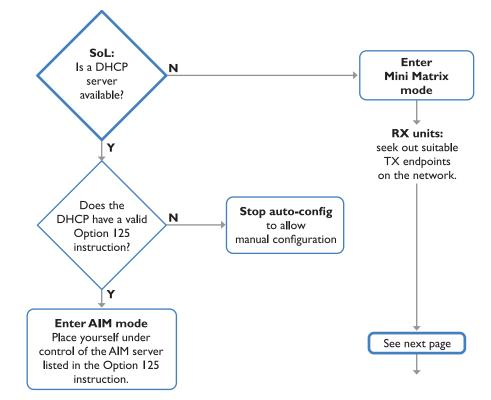
Note: If an AIM server is present on the network then the modules don't have to be within SoL procedure for it to be placed under AIM control.
