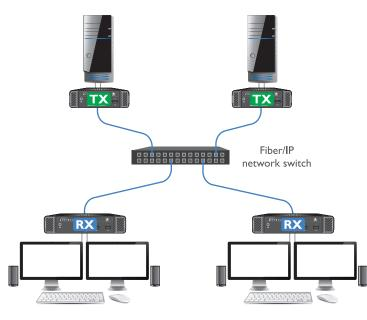
This method of connection works well for small numbers of TX and RX units, but will become more difficult to manage as more units are attached. The maximum number of TX sources that can be made available to any RX is sixteen.
