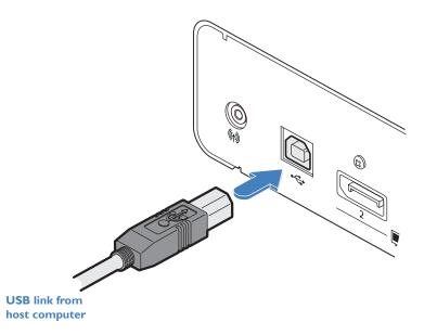
2 Connect the type A connector of the supplied cable to a vacant USB socket on the host computer.
