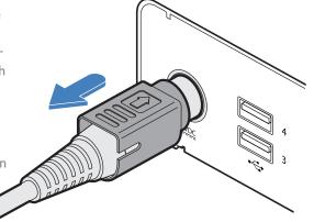
Gently pull back the plug outer body to release the lock
