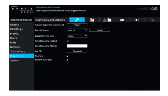
**Perform IGMP Test** - Allows you to conduct an IGMP test on connected devices, selectable from the drop-down list.
