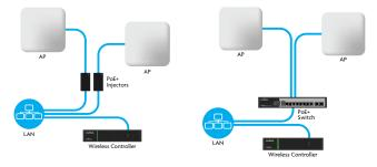
Access Point Placement: Place APs to ensure adequate coverage, but not so far apart that there is no signal overlap. You may have to experiment with AP placement to optimize the roaming experience. The APs should overlap enough that the client device has a good connection to the AP to which it is currently attached, but also sees the next-nearest AP.
