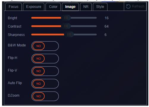
**Note:** Flip-H and Flip-V are only available when Auto Flip is disabled. DZoom allows the camera to digitally zoom in on a shot past the standard optical zoom range but may reduce image quality.
