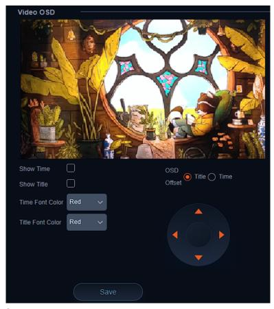
Video OSD or On Screen Display gives users the option to display the Device Name, Date, and Time, on the stream of the camera. This can be useful in easily identifying cameras when multiple are in use simultaneously in a production or security type setup.
