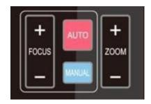
**FOCUS** + (near) : Press to adjust the lens focus.
