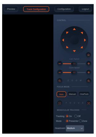
To set up or enable auto-tracking, select "Track Configuration" on the top right corner.
