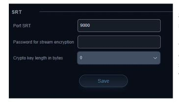
**SRT** is an alternative to standard RTSP streams. SRT can recover from packet loss of up to 15%. This provides a better video stream on substandard or congested networks. It also helps keep streams secure and easily travers firewalls.
