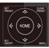
Set Preset: Press the [SET PRESET] button, then press the number buttons 0-9 to set the preset positions.
