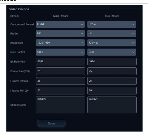
From the Video Encode tab users can edit the following parameters for the main and sub streams:
