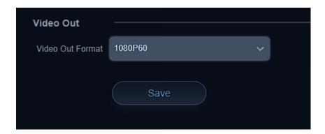
Video Out is used to adjust output resolution of the camera to its physical HDMI and SDI outputs.
