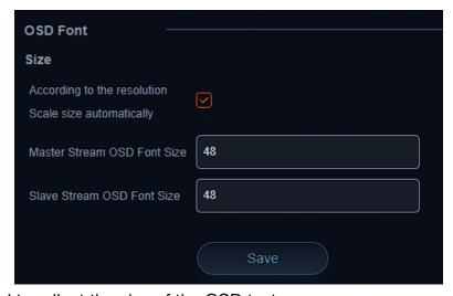
OSD Font is used to adjust the size of the OSD text.
