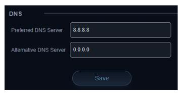
Allows users to change the Prefered and Alternate DNS server settings of the camera to a specific DNS server of their choice if required by their network.
