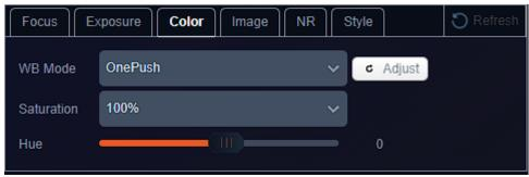
Press the "Adjust" button to lock in new white balance settings. This setting is useful when a white balance card is used.
