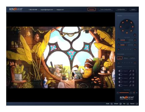
After successfully logging into the management interface, the web portal will enter the "Preview" tab. In Preview, users can control pan/tilt, zoom, focus, video capture, sound, focus, full screen preview, as well as set and recall preset positions and configure the "Home" preset position.
