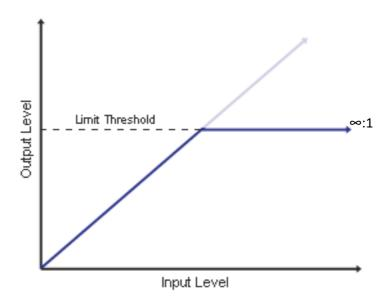
**Threshold** (-6 - +24 dBu) is the signal level at which the limiter will be activated. Setting it to OFF disables the limiter.
