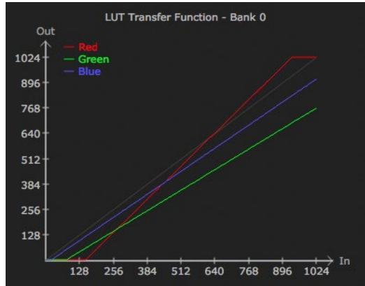
Figure 13. Example LUT Transfer Function Curves
