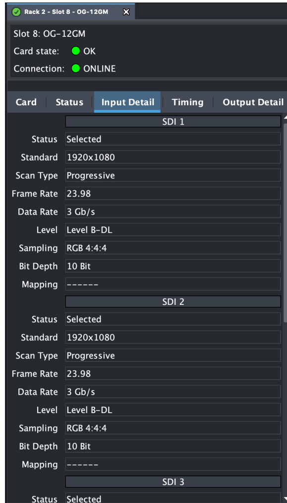
Figure 13. Example of Input Detail Tab Screen in DashBoard reflecting Quad 3G-SDI to Single 12G-SDI conversion using Square Division (Quadrant) to Two Sample Interleave (2SI) pixel mapping.
