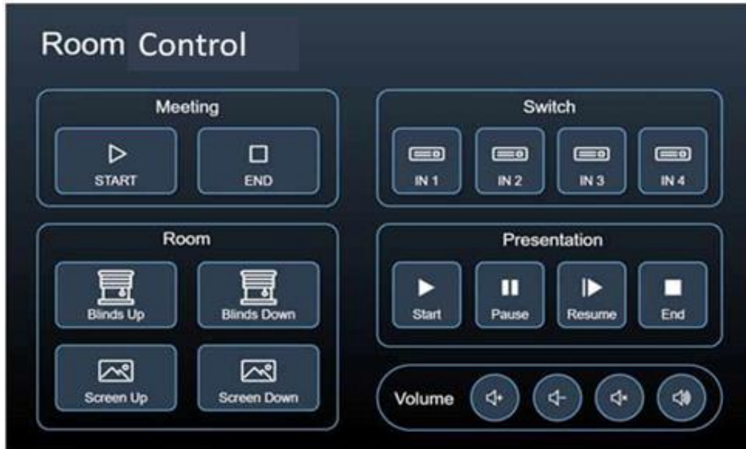
Figure 10: Default Kramer Aware Room Control Panel
