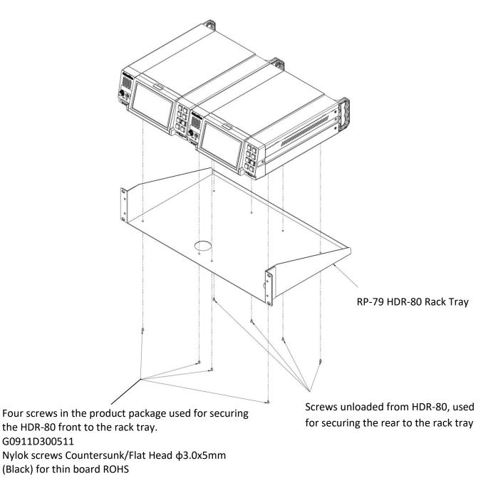
There are four extra G0911D501011 Nylok screws Round Head with spring washer M5x10mm (Black) for securing HDR-80 to the rack tray.
