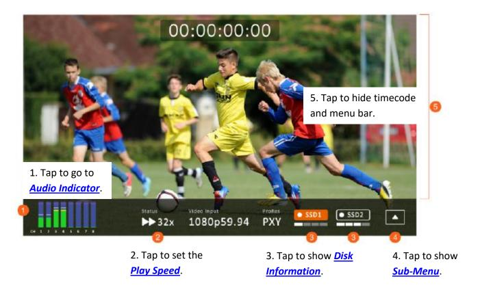
In the full screen mode, you can either press the **Play/Pause** button to play the record clip or press the **Record** button  $\rightarrow$  **Play/Pause** button to start recording.
