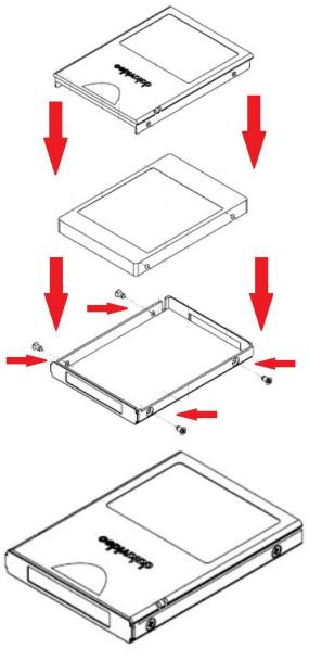
2. As shown in the diagram on the left, place an SSD in the drive enclosure then re-secure the top plate of the drive enclosure using the four screws removed earlier.
