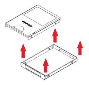
1. Remove the four screws on two sides of the SSD disk enclosure then lift the top plate.
