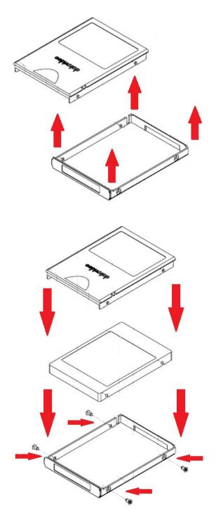
1. Remove the four screws on two sides of the SSD disk enclosure then lift the top plate.
