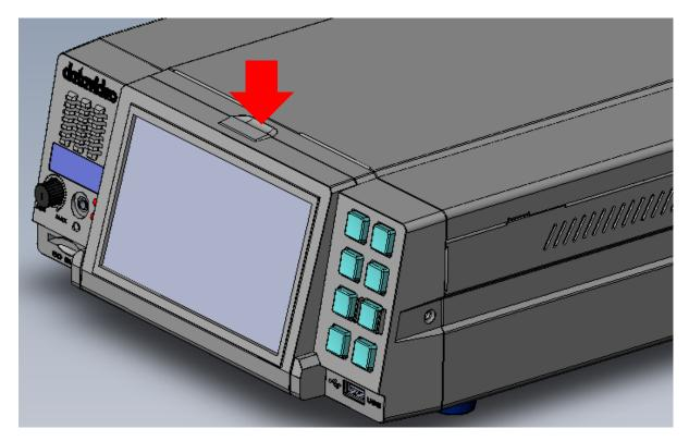
To flatten the 5" touch screen, first press the latch indicated by the arrow in the diagram above then pull the screen forward, after which you should see two SSD slots as shown below.
