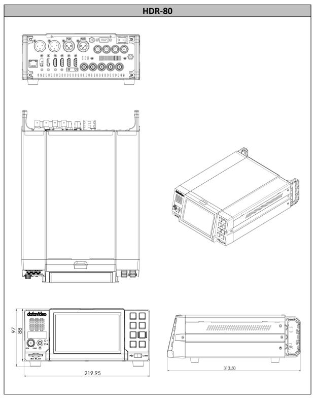
All measurements in millimeters (mm)
