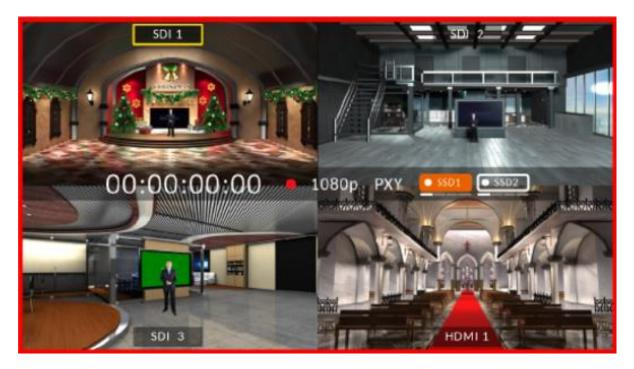
On the quad split screen, tap one of the screens to switch between HDMI and SDI video sources.
