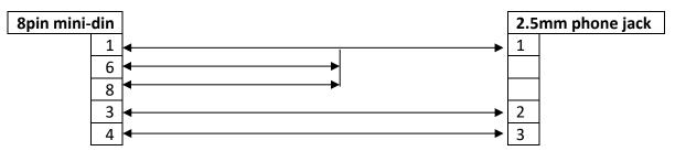
Warning: The 8pin snap-and-lock mini-din connector of the remote cable will be securely fastened once plugged into the Remote port. To remove, use two fingers to gently hold the part of the plug labelled by two arrows then pull the connector outward.
