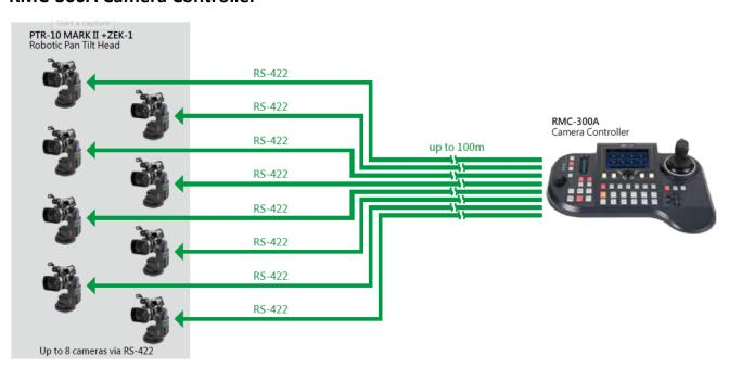
To control the camera mounted on PTR-10T MARK II using the camera controller, first connect one of the RJ-45 ports provided on the controller rear to PTR-10T MARK II's RS-422 IN port via an RJ-45 cable. Then depending on the protocol used, either connect PTR-10T MARK II to the camera via the Remote port (LANC/BX-Lens) through a remote cable or via the RS-232/422 OUT port (RS-232/RS-
