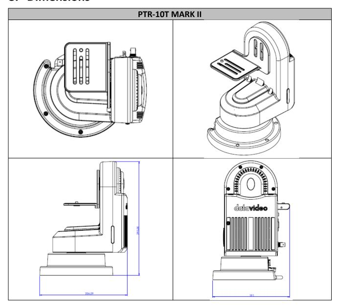
All measurements in millimeters (mm)
