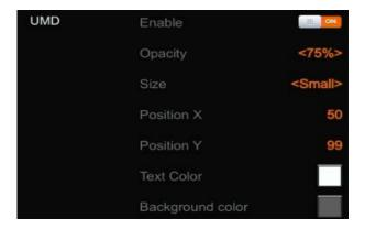
The UMD string content for the 4 HDMI inputs can be set from the menu. Users can rename the UMD content for each window by using a virtual keyboard and rotary button. It supports a maximum of 10 characters for the UMD content. In the example below the input has been renamed from HDMI 1 to CAM1.
