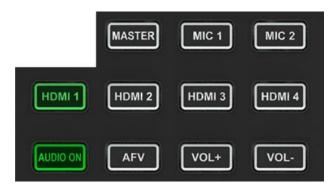
When any button in Part-A is pressed and the indicator for the button in Part B turns green it means the corresponding audio function is ON. When the indicator is OFF it means the corresponding function is OFF.
