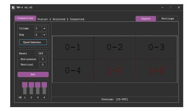
For each connected device, VW-4 App also enables performing factory reset, upgrading the firmware, viewing network settings and copying the EDID to the input from a selected EDID source.
