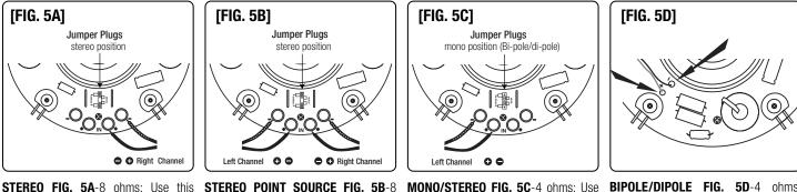
configuration to drive one channel (left OR right) of a stereo pair. Set jumper plugs in the stereo position. Connect the right or left signal wire to the right set of terminals on the rear of the speaker.
