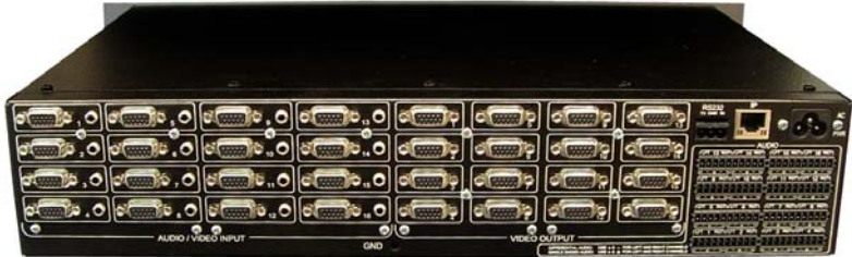
Figure 1 – Rear panel of the standard matrix showing all the connections
