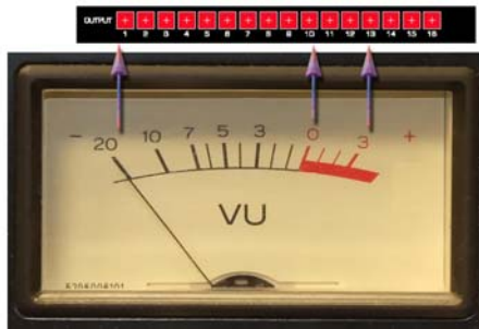
Figure 12 –Comparison with Analog VU meter on a 16x16 Matrix
