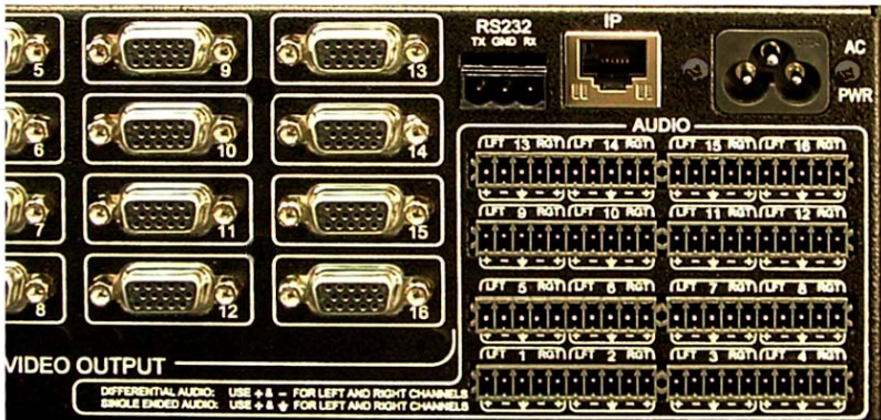
Figure 4 – Standard matrix audio and video outputs
