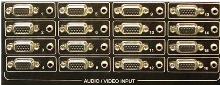
Figure 2 - Audio and video inputs on Standard 16x16 unit
