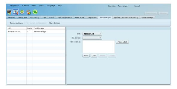
Alarm Settings: Set up alarm range for temperature and humidity. If detected figures are out of setting range, it will send alarm message.
