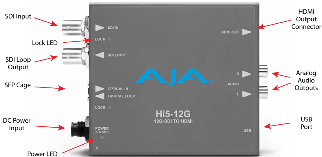
Figure 2. Hi5-12G Converter Connections
