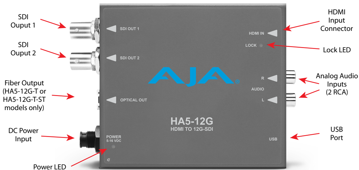
Figure 2. HA5-12G/HA5-12G-T Converter Connections
