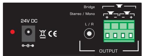
Power input jack is used to connect the supplied 24 v adapter. There is a Red LED indicator to show power status.
