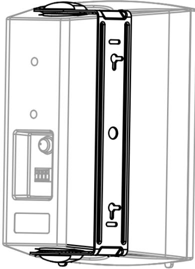
Figure 3: Yarden 6-O with Brackets Connected
